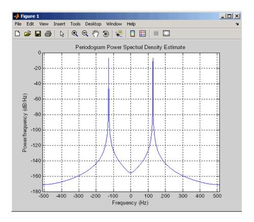
Notice that the peaks of this plot are not the same height as the mean-square spectrum peaks plotted above. The area under the PSD curve is the measure of the average power, not the peak heights. By using the avgpower method and converting the result to dB, you can see that the average power is the same for both of them.
