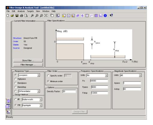
The bottom half of FDATool shows the Filter Design panel, where you specify the filter parameters. Other panels, such as Import filter from workspace and Pole/Zero Editor, which you access with the buttons on the lower left, are also displayed in this area. If you have other products installed, you may see additional buttons.
