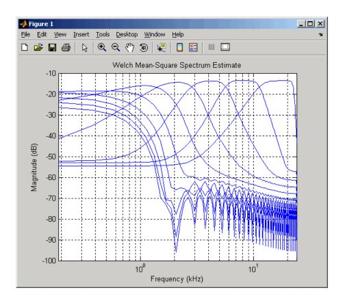
The syntax for using psd, msspectrum, or pseudospectrum is the same. As shown in the example above, the first input is the spectrum object (h) and the second input (yw) is the signal to measure, followed by any settable properties using property-value pairs (e.g., 'Fs', Fs). To set property-value pairs, you list the property first and then the value for that property.
