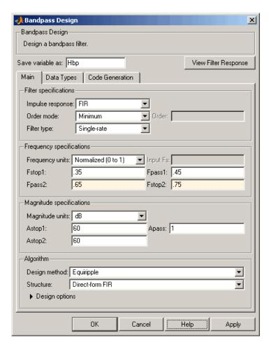
**3** Enter the correct frequencies for **Fpass2** and **Fstop2**, as shown in the preceding figure, then click **OK**. Here the specification uses normalized frequency, so that the passband and stopband edges are expressed as a fraction of the Nyquist frequency (in this case, 48/2 kHz). The following message appears at the MATLAB prompt:
