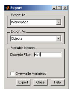
4 Repeat steps 1 through 3 for each of the remaining nine filters. Highlight each filter individually to make it the active filter and change the **Discrete** Filter name to match the filter number. When you finish you will have 10 dfilt objects in the workspace.
